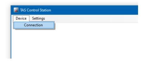
**Connecting** - Open the connection dialog and select the appropriate port identified by USB and the device ID/serial number which is located on the back of the interface modules at the bottom of the label. (Note: Windows can take a few seconds to instantiate the device when it is not already in memory so there may be a short delay in populating the port in the connection dialog).
